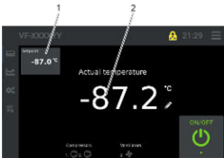
Fig. 101: Cooling chamber temperature set point icon
