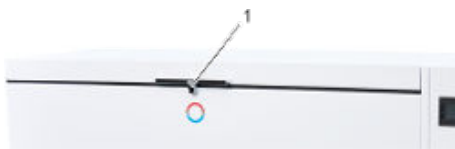
Fig. 12: Refrigeration compartment lock
